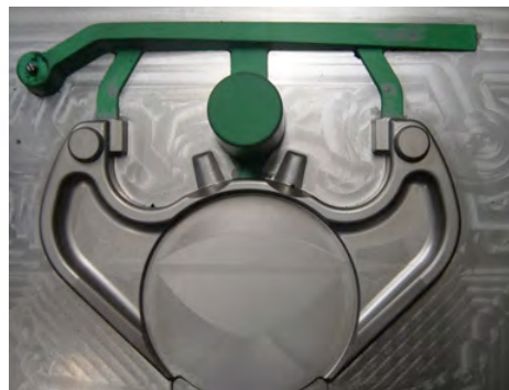
Figure 7. Photo of revised pattern with single feeder.
