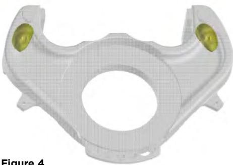
Figure 4. Areas of high modulus value in the casting.
