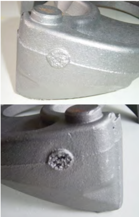
Figure 3. Feeder contacts with original design (2 feeders).
