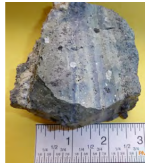
Figure 4. Insoluble buildup removed from Foundry G's coreless induction furnace after 48 hours of operation.
