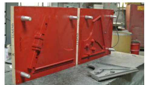
3D printed ABS pattern mounted for sand casting — Photo courtesy of Titan Robotics
