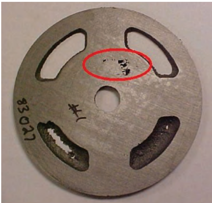
Figure 1. Slice through the left casting, showing shrinkage
