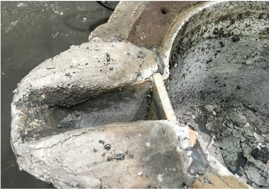
Open Back Teapot Spout: Shows how the teapot spout is created by inserting a refractory board
