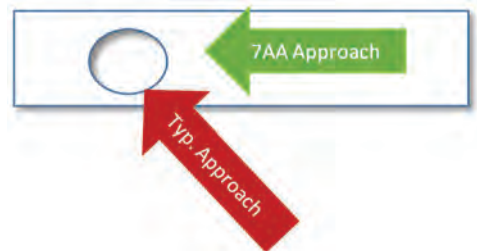
Figure 4: Example approach paths to the pour hole on the shot sleeve, 7AA vs. typical path
