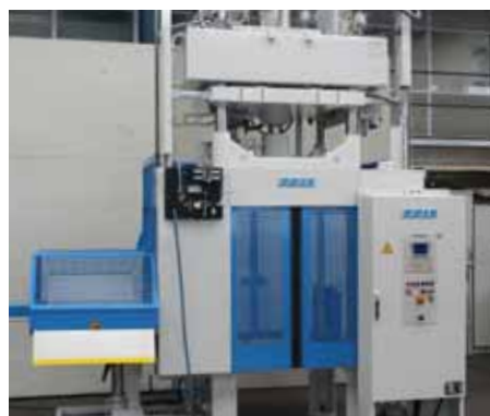
The Reis trim press SEP in three-column design can be set reliably and quickly.
