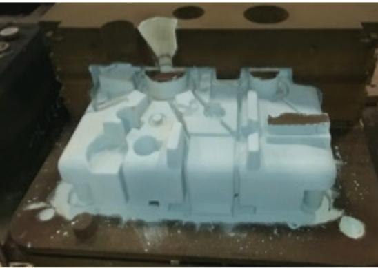
Figure 2: Partially assembled 3D printed mold
